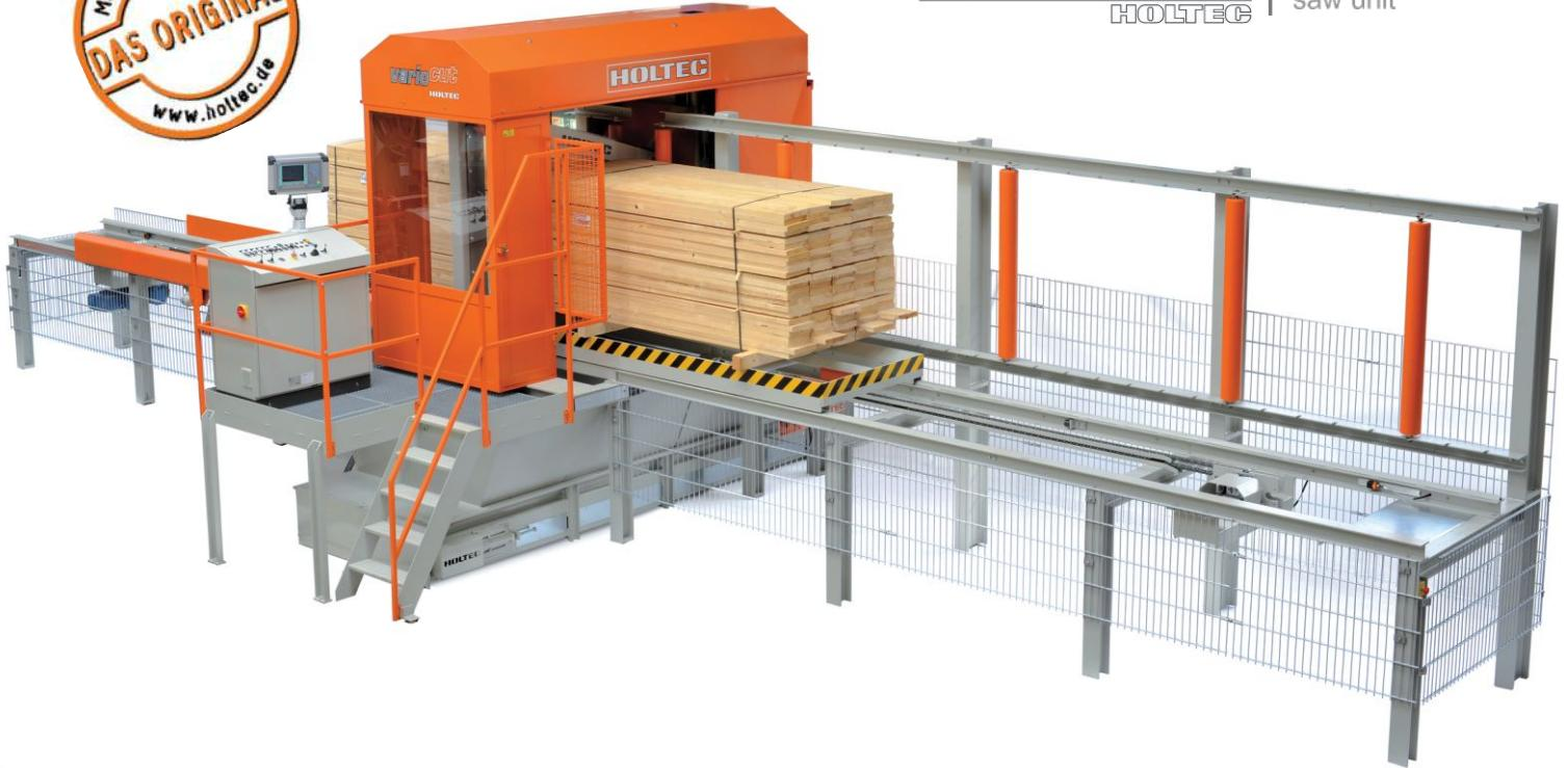
Package crosscut saw Vario-Cut with moveable carriage and stationary saw unit. The packages are positioned by means of an electrically controlled carriage. During the cutting process the guide bar can be guided through the package in an angle of 0-15°. The cutting of partial packages is possible on any package height. By means of the parallelogram set-off device the cutting kerf can be opened - condition for optimally carrying out multiple cuts within one package.
